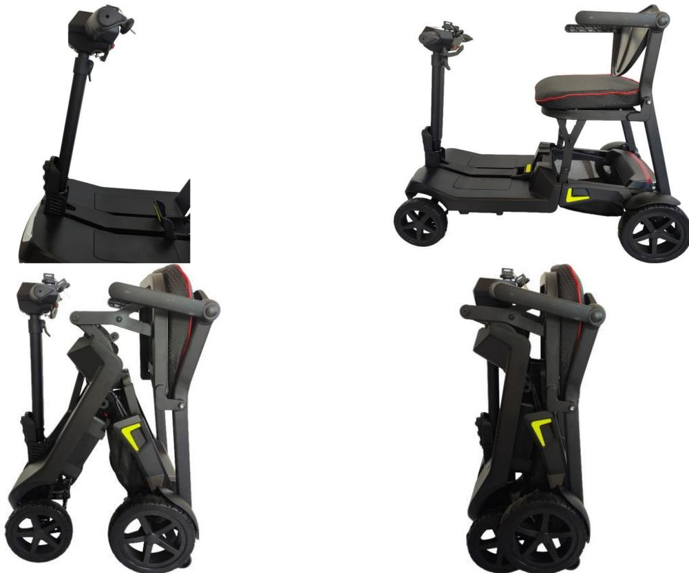
Fig 10. Disposition steps of scooter
