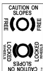
At the rear of the **Mobility scooter YL-985S** is the manual release lever of the EMB. When using this lever, be careful not to touch the surface of the motor, as it could be very hot and cause injury. See the warning label at the rear of the scooter near the lever.
