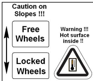
Do not release either the manual or the manual release lever of the electromagnetic brake (EMB) when the **Mobility scooter YL-985S** is on a slope. When on any sort of an incline, never place the **Mobility scooter YL-985S** in freewheel mode while seated on it or standing next to it.
