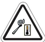
When removing the battery cover, watch out for hot parts. The motor, axle, EMB, electronic cards and electronic controller might be hot, Do not touch them until you have checked their temperature.
