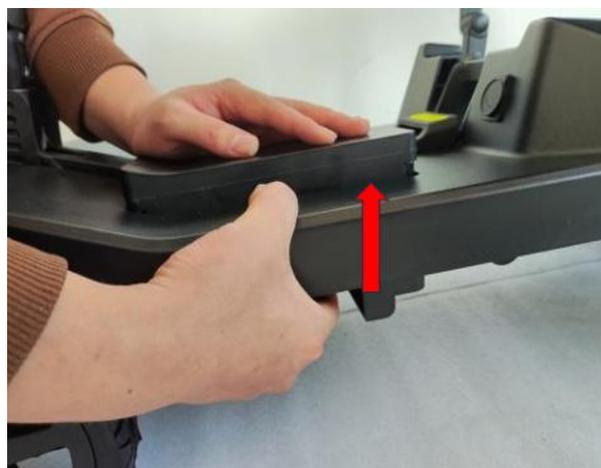
Fig 9. Battery box removal
